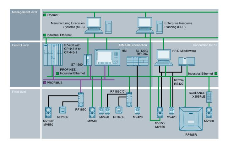
The following communication options are available for connecting SIMATIC MV optical readers to the automation or IT level:
