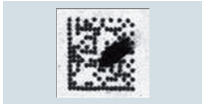
Damaged surface of the marking or part
