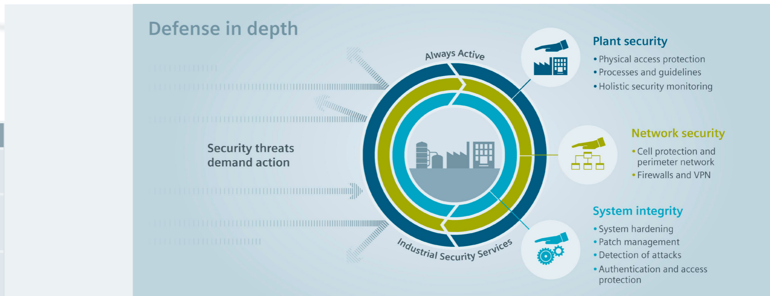
Network security as a central component of the Siemens industrial security concept
